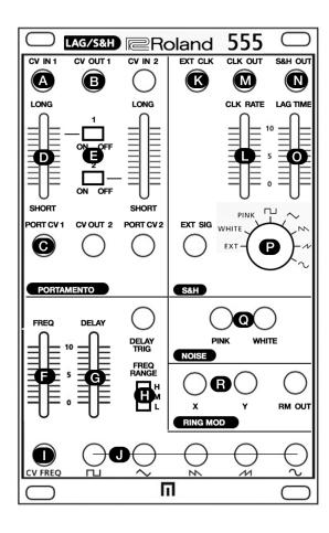
A PORTAMENTO CV IN 1/2 Input point for the signals to which to apply portamento.
