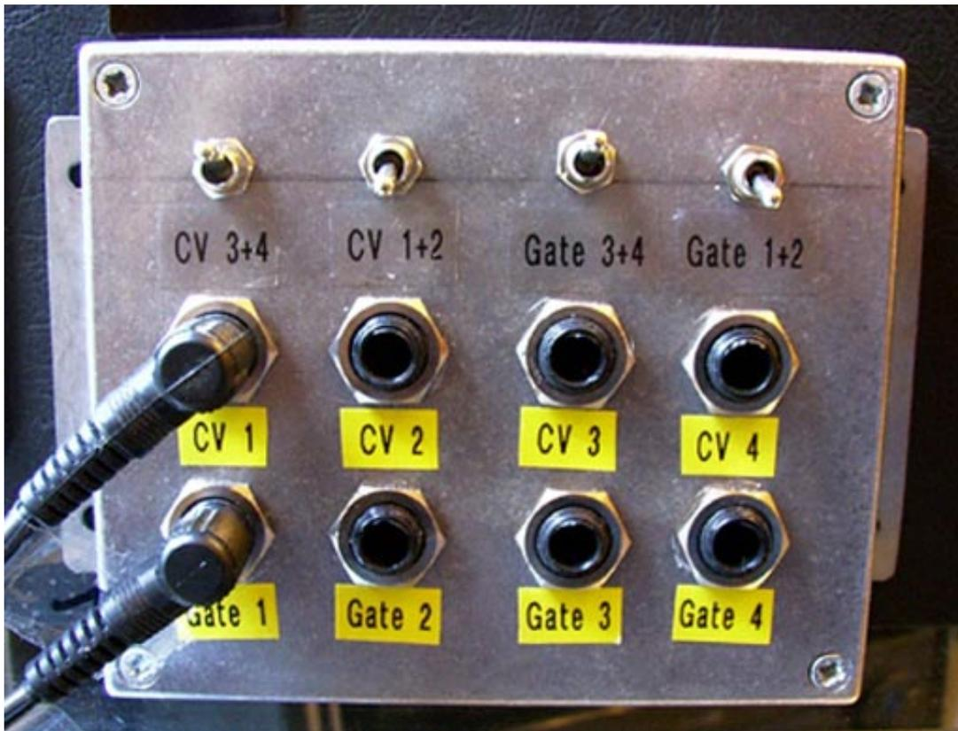
This layout enables the user to control the Gate signals externally and the CV signals via keyboard or vice versa. Jupiter's arpeggiator is thus fully utilizable and, at the same time, can be combined with the external signal controls. The arpeggiator's already-present external sync IN takes care of the right timing.
