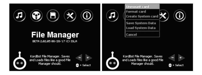
The KordBot uses an SD card as an external storage drive. With the File Settings menu, the user can mount or unmount the drive, format a new SD card, create a system disk and save and load the entire configuration of the unit. SD cards of 2 and 4 Gigabytes are supported. Users may use 8 Gigabyte cards, but the SD driver limits storage to 4 Gigabytes, which should be enough room for a lot. A lot a lot.Lots of a lot.
