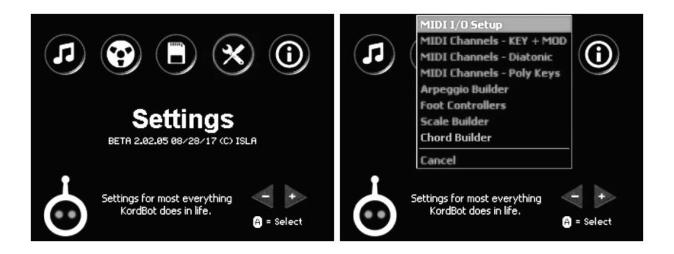
The Settings menu allows the user to configure much of the KordBot to tailor the system as desired. MIDI Input/ Output routing and channel set ups for individual keys, banks or segments of banks is available here.
